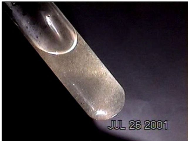
Distilled Concentrate of Rain Water in Test Tube. Metallic particulates are highly visible.
